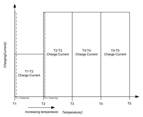
Figure 2-7. Temperature Hysteresis for Charging Current
