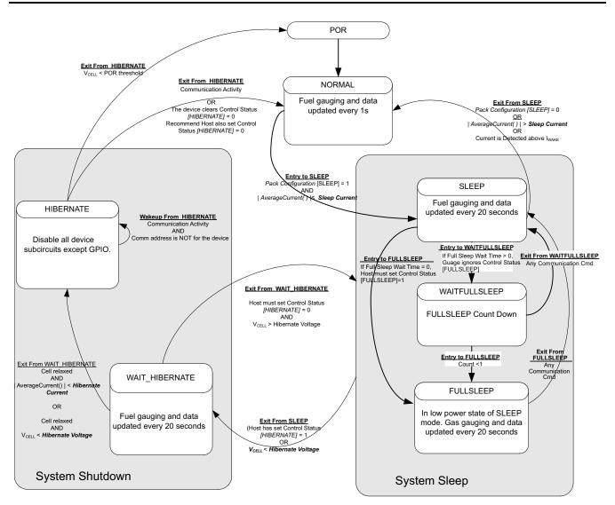
Figure 2-9. Power Mode Diagram—System Sleep
