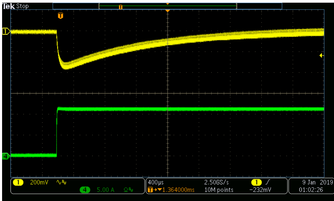
Figure 12. Load Step Up With 40 V IN
