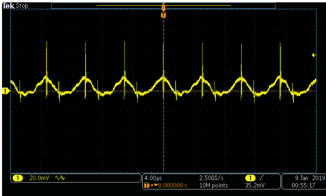
Figure 8. Output Voltage Ripple 40 V IN
