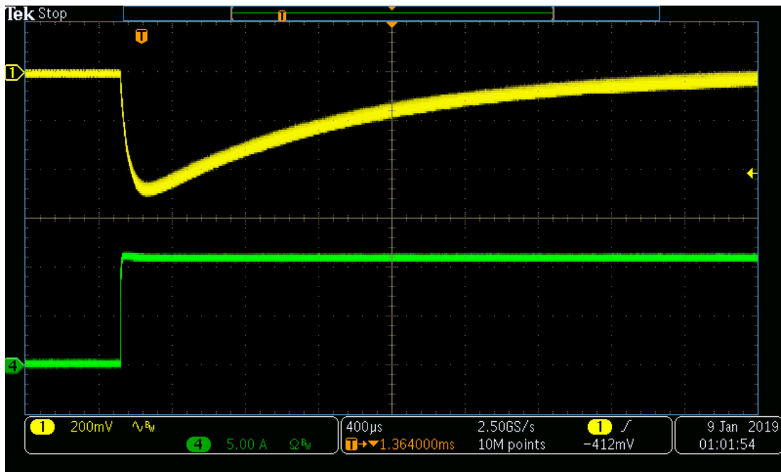
Figure 10. Load Step Up With 20 V IN
