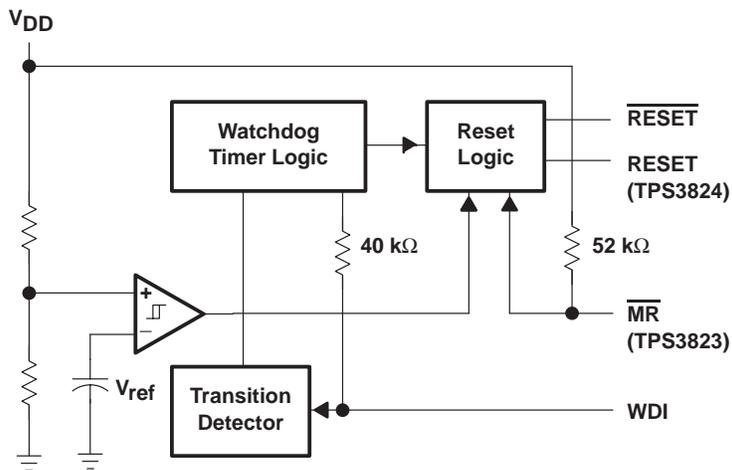
Figure 3. Simplified Block Diagram
