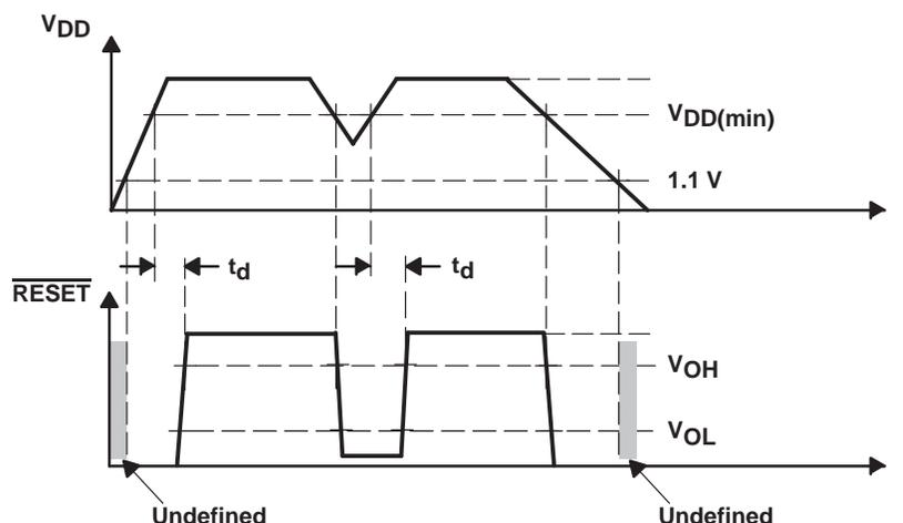
**Figure 5. Timing Diagram of V<sub>DD</sub> and  $\overline{\text{RESET}}$  Output**
