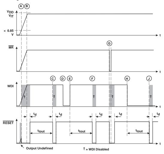
Figure 14. Watchdog Circuit Timing
