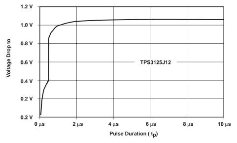
Figure 11. TPS3125J12—Reaction fo Voltage Drops
