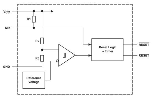
Figure 5. TPS3125 Supply Voltage Supervisor
