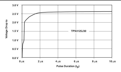
Figure 12. TPS3125J30—Reaction fo Voltage Drops
