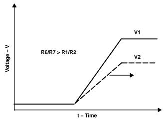
Figure 5. Ratiometric Sequencing With V1 Rising Before V2
