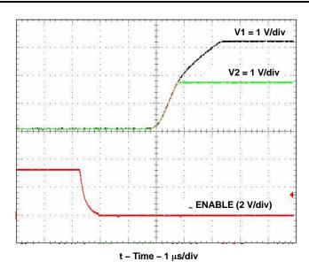
Figure 2. Power-Up Waveform With Simultaneous Tracking
