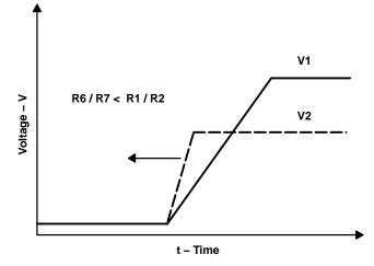
Figure 4. Ratiometric Sequencing With V2 Rising Before V1
