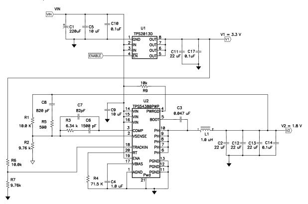
Figure 1. TPS54380 With TPS2013 Distribution Switch
