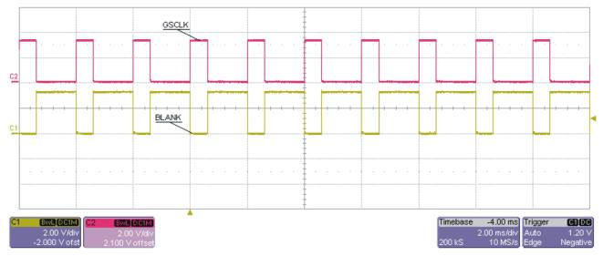
Figure 5. TLC5940 PWM Dimming
