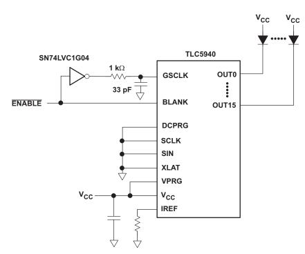
Figure 2. TLC5940 Controlled With One PWM/ENABLE Signal
