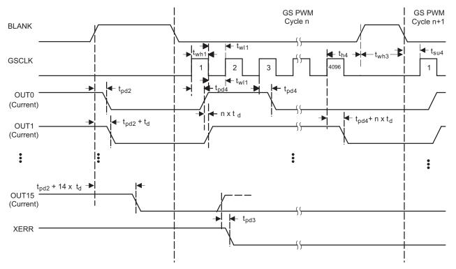
Figure 3. TLC5940 Grayscale PWM Cycle Timing Chart
