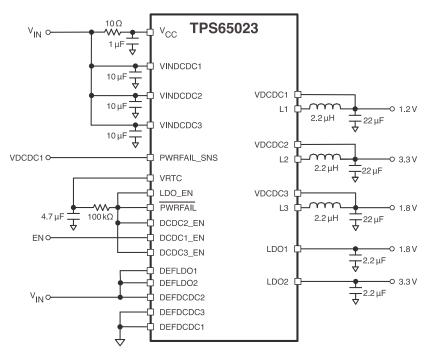
Figure 3. Sequencing Schematic
