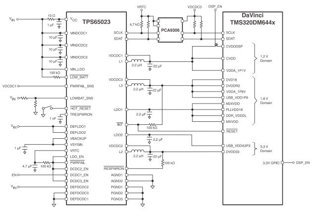
Figure 5. Full Schematic for Sequencing and Reset
