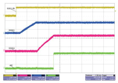
Figure 6. Scope Trace of INT Signal for DaVinci™ Reset
