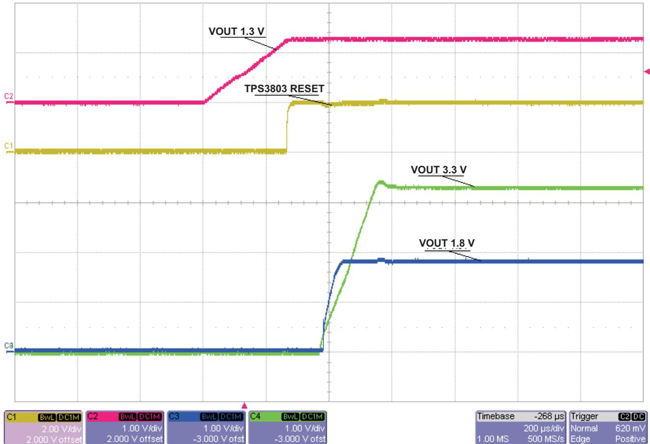
Figure 5. Power-Up Sequence Showing TPS3803-01 RESET Signal
