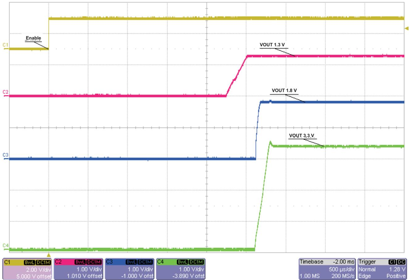
Figure 2. Power Up With 2-V Input and ENABLE Voltage
