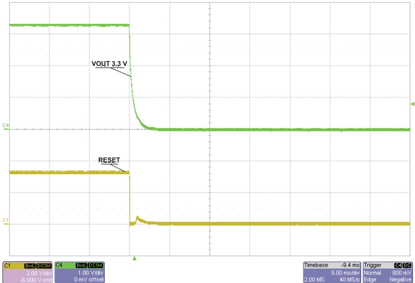
Figure 6. Power-Down Sequence Showing TPS3808G33 RESET Pin Signal
