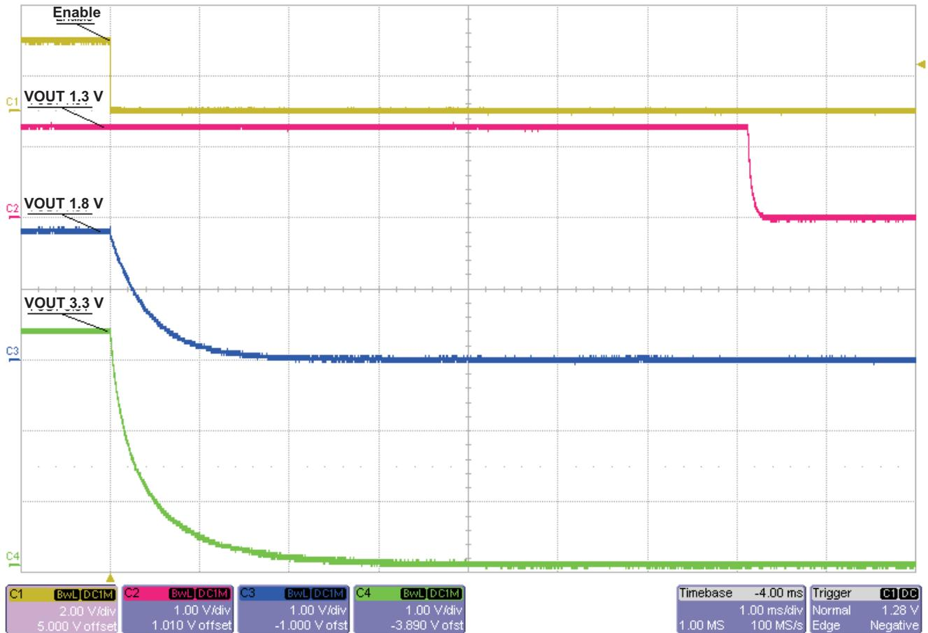
Figure 4. Power Down With 2-V Input and ENABLE Voltage
