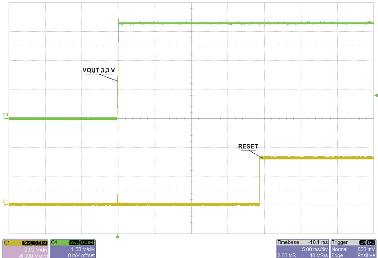
**Figure 3.  $\overline{\text{RESET}}$  Pin of TPS3808G33 Pulled High**
