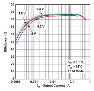
Figure 3. Efficiency vs Output Current (TPS65053)
