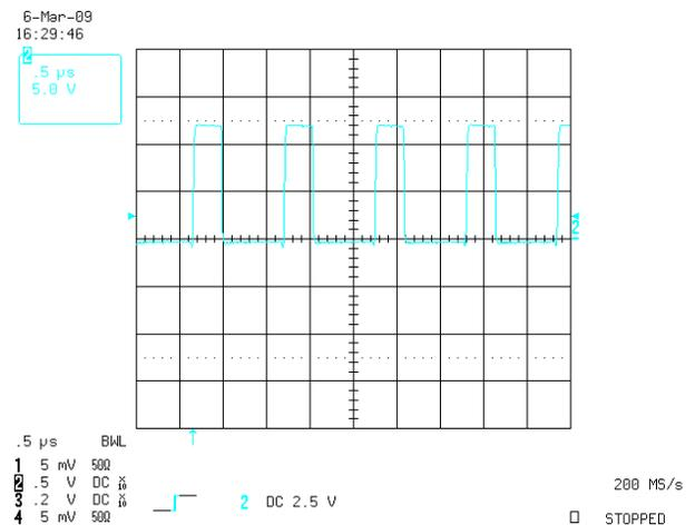
Figure 9. Switching Node Waveform,  $V_{IN} = 12\text{ V}$
