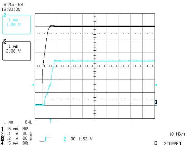
Figure 4. Startup  $V_{IN} = 12\text{ V}$ ,  $I_{LOAD} = 1.5\text{ A}$
