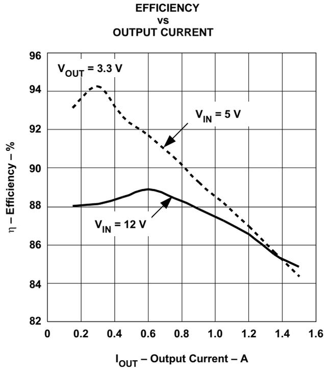
Figure . Figure 10. TPS62111 Efficiency
