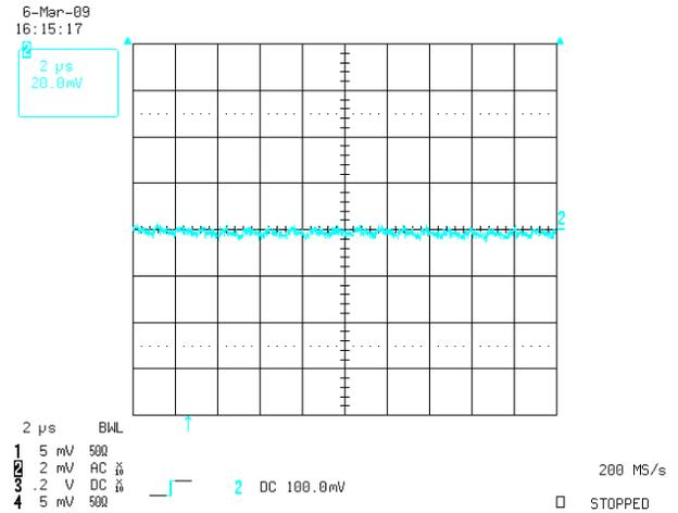
Figure 7. Output Ripple Voltage,  $V_{IN} = 12\text{ V}$
