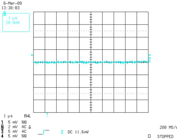
Figure 6. Output Ripple Voltage,  $V_{IN} = 5\text{ V}$
