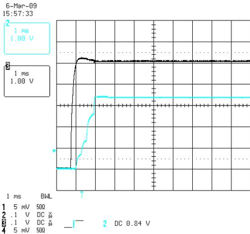
Figure 2. Startup  $V_{IN} = 5\text{ V}$ ,  $I_{LOAD} = 1.5\text{ A}$
