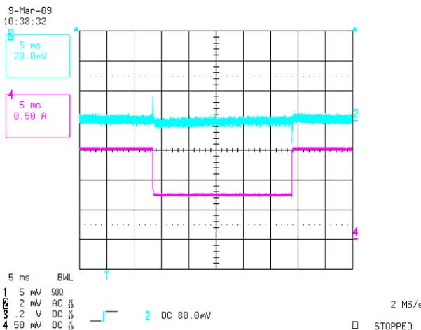
Figure 8. Load Transient Stepped Between 750 mA and 1.5 A,  $V_{in} = 12\text{ V}$
