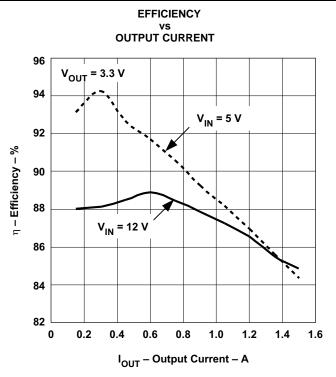
Figure . Figure 10. TPS62111 Efficiency
