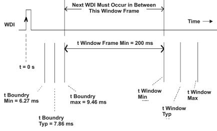
t Boundry Max + t Window Min = 9.46 ms + 200 ms = 209.46 ms
