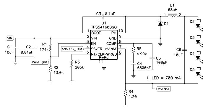
Figure 1. LED Driver Circuit
