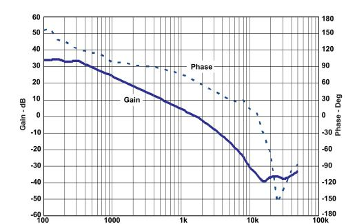
Figure 3. Type I Compensation Closed-Loop Response
