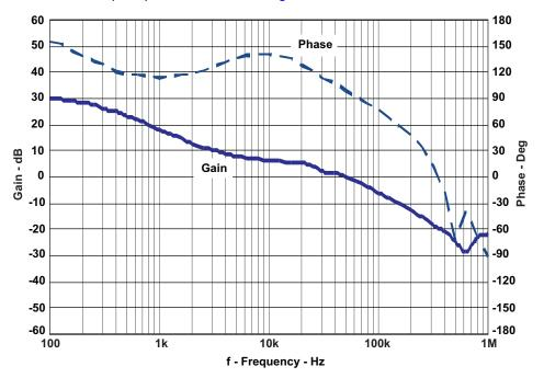
Figure 4. Type II Compensation Closed-Loop Response
