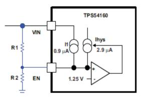
Figure 2. Adjustable Undervoltage Lockout
