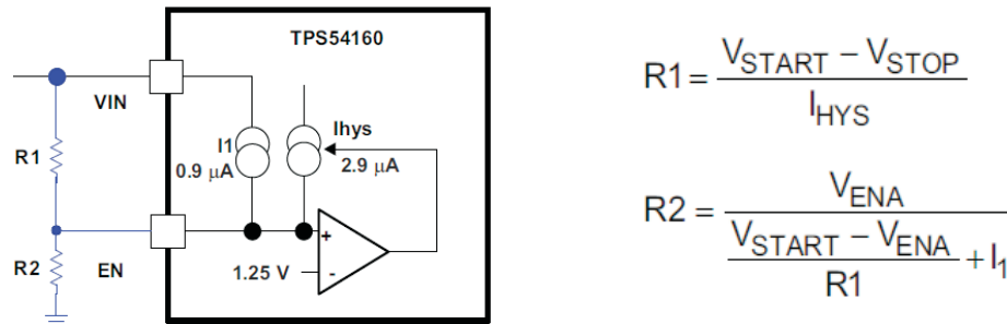
Figure 1. Adjustable Undervoltage Lockout
