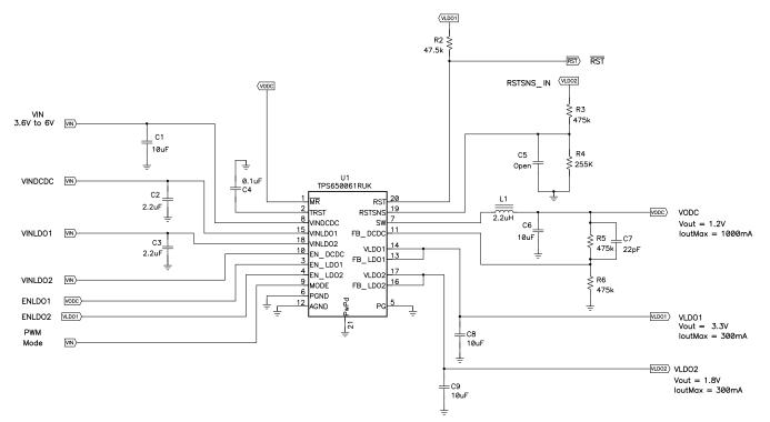
Figure 2. TPS650061 Schematic Diagram
