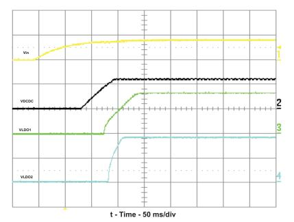
Figure 3. TPS650061 Power Up – Ch1-Vin, 5 V/div; Ch2-VDCDC, 1 V/div; Ch3-VLDO1, 2 V/div; and Ch4-VLDO2, 1 V/div
