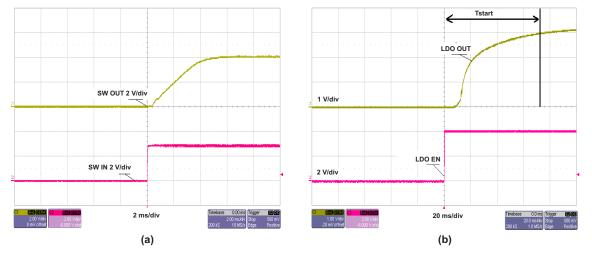
Figure 6. Switcher and LDO Output Voltage Turnon, LDO Enable With  $C_{NR}$  = 100 nF
