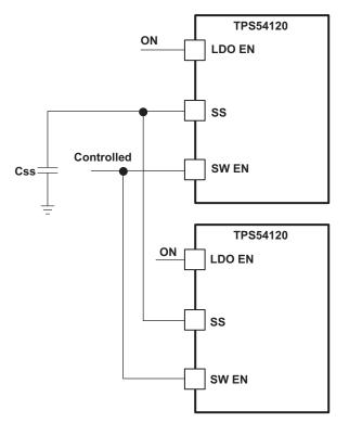
Figure 13. Ratiometric Start-Up Using SS Pins and Enabling Switcher
