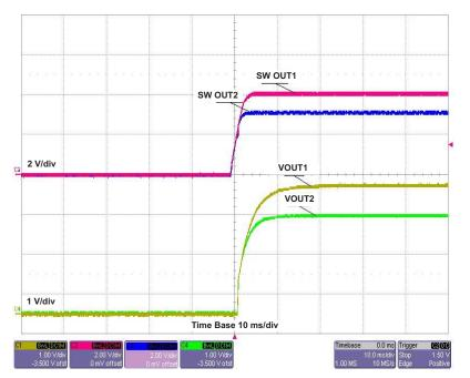
Figure 18. Simultaneous Start-Up
