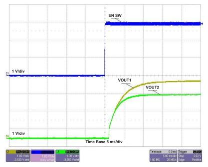
Figure 14. Ratiometric Start-Up Result of Circuit in Figure 13
