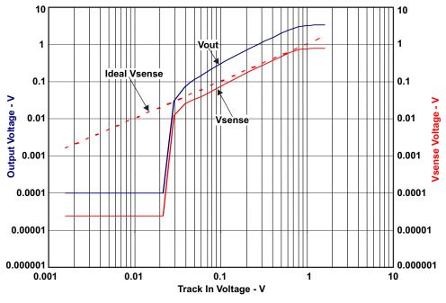
Figure 2 shows the relationship between the tracking voltage with the output voltage and the sense voltage of the switcher.
