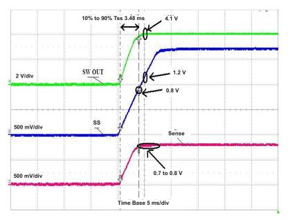
Figure 3. Slow-Start, Ramp-Up Time of Switcher
