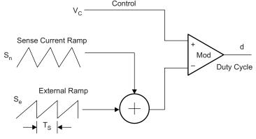
Figure 6. PWM with Slope Compensation
