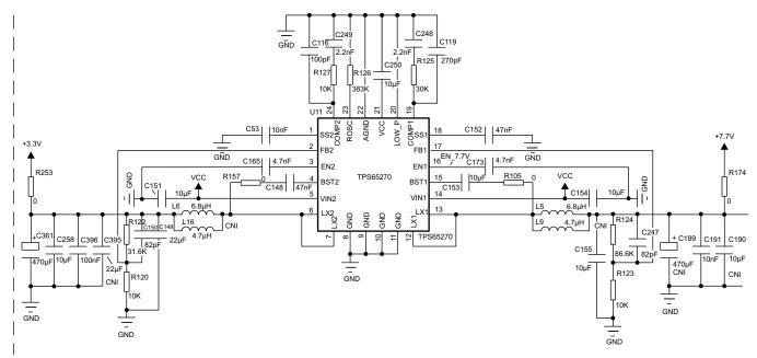
Figure 11. TPS65270 Design with 3.3- and 7.7-V Output
