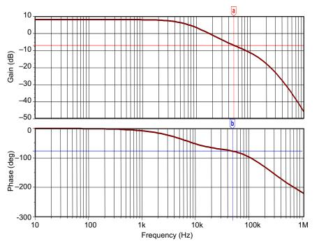
Figure 16. Bode Plot of Control to Output
