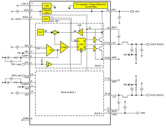
Figure 1. TPS65270 Block Diagram
