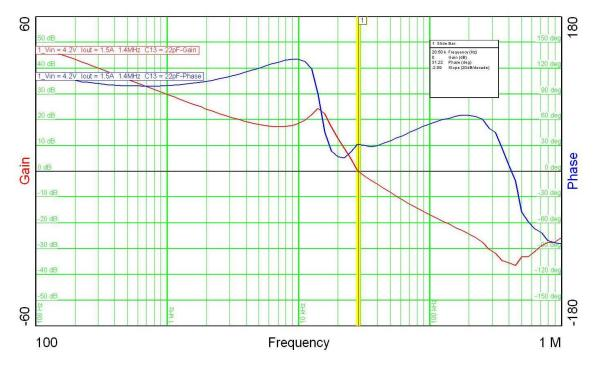
Figure 5. Control Loop Gain with 2.2-µH Inductor and 100-µF Capacitor
