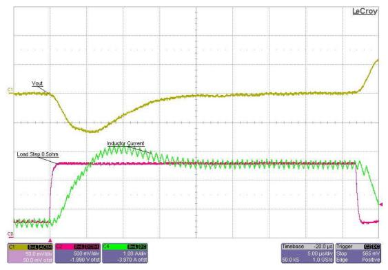
Figure 3. Load Transient with 2.2-μH Inductor and 100-μF Capacitor
