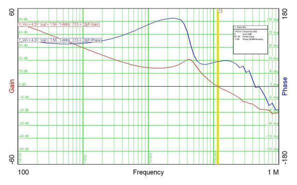
Figure 4. Control Loop Gain with 2.2-μH Inductor and 10-μF Capacitor
