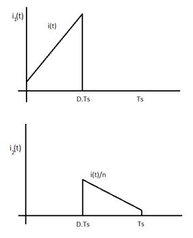
Figure 4. Current Waveforms for the 2-Port Network
