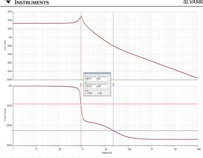
**Control-to-Output Transfer Function Plotted using Tlna** Figure 8.
