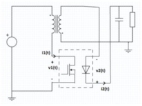
Figure 2. Separating Out the Non-Linear Switch Elements
