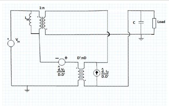
Figure 6. Complete Linear Circuit for Flyback Converter
