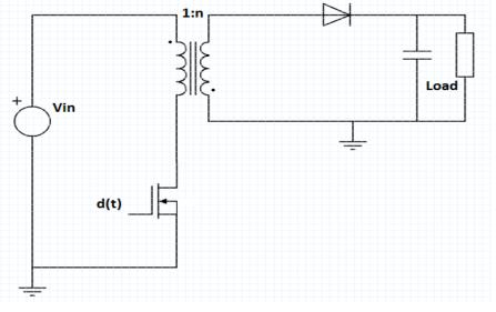
Figure 1. Basic Topology of a Flyback Converter
