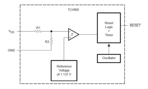
Figure 2. Functional Block Diagram
