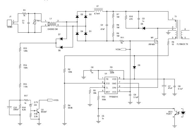
Figure 4. Input Over-Voltage Protection With Conventional Approach
