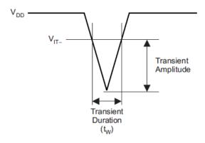
Figure 6. Voltage Transient Measurement
