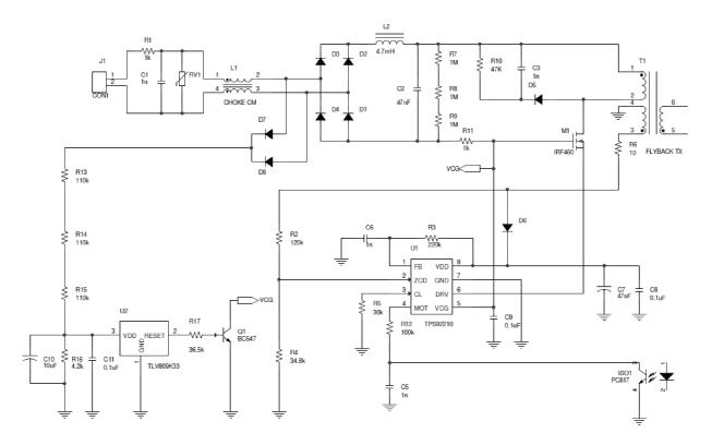
Figure 5. Input Over-Voltage Protection With Voltage Supervisor
