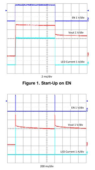
Figure 2. PWM Dimming on EN With 1% Duty Cycle at 1 Hz
