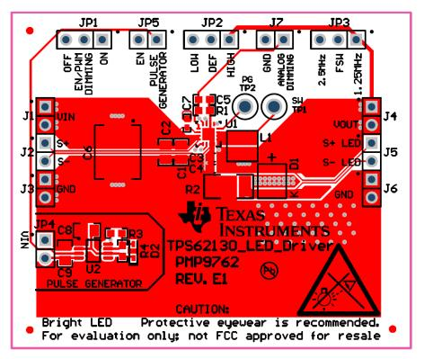
Figure 7. Assembly Layer
