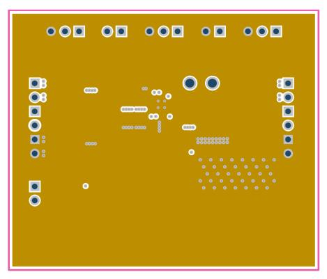
Figure 9. Inner Copper Layer 1
