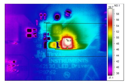
Figure 5. Thermal Performance (1-A LED Current, DC)
