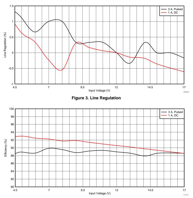
Figure 4. Efficiency vs Input Voltage
