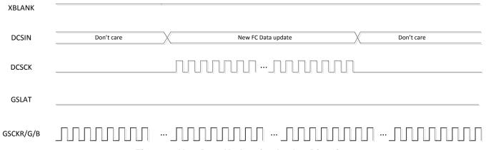
Figure 4. New Data Update for Analog Dimming
