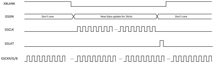
Figure 3. New Data Update for PWM Dimming
