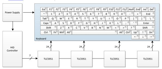
Figure 1. TLC5951 Multi-channel LED Driver for Keyboard Backlighting Application Drawing
