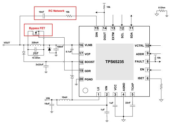
Figure 21. Application for DiSEqc2.x Support on TPS65235
