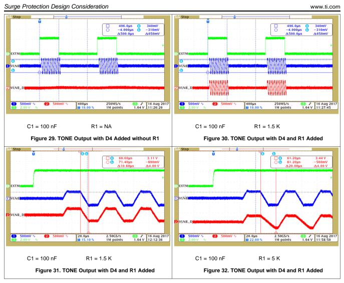
The smaller R1, the more power loss, but the larger R1 cannot provide enough discharge current for C1 to discharge in time, to meet the tone spec requirement for falling edge. To choose the suitable R1, use Equation 5.
