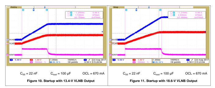
For TPS65233, all the behaviors are same with the TPS65235, while the hiccup ON time is fixed about 4 ms. To support lower OCL setting or higher capacitive load on VLNB output, if hiccup happens when startup, the larger TCAP capacitor  $C_{SS}$  should be used to decrease the startup current lower than OCL value.
