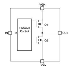
Figure 2. Level Shifter Channel Without Gate Voltage Shaping
