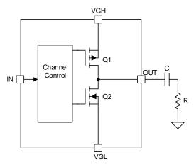
Figure 3. Level Shifter Channel With Load
