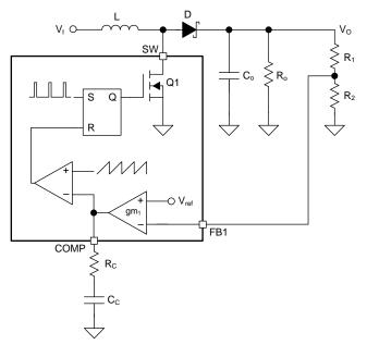
Figure 1. High-level Scheme Voltage-Mode Control
