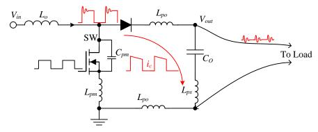
Figure 2. Simplified Boost Converter and Operating Waveform
