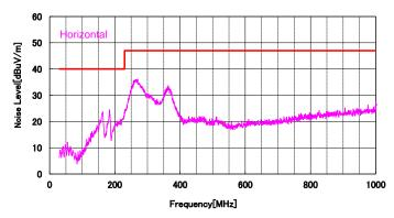
Figure 8. Radiated Noise With Bead and RC Snubber
