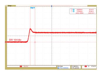
Figure 5. SW Waveform With RC Snubber
