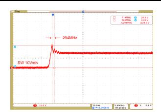
Figure 3. SW Waveform at V<sub>IN</sub> = 7.8 V, V<sub>OUT</sub> = 16 V, I<sub>OUT</sub> = 2 A
