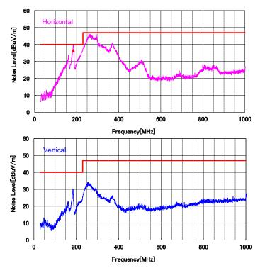
Figure 1. TPS61178EVM Radiated Noise
