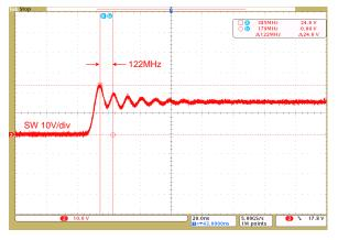
Figure 4. SW Waveform With 820 pF
