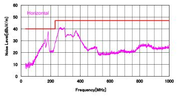
Figure 6. Radiated Noise With the RC Snubber
