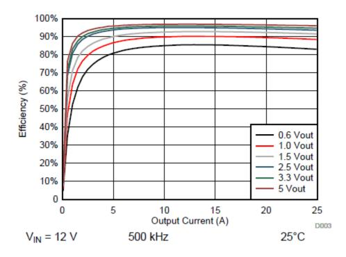
Figure 5. TPS543B20 Efficiency Plot
