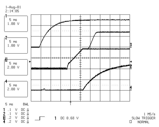
Figure 2. Output Voltage Waveform for Sequential Start-up: Channel 1: 3.3 V; Channel 2: Vcore; Channel 3: PG; Channel 4: Input Voltage
