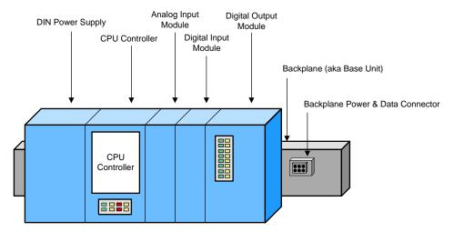
Figure 1. Typical PLC System with a Backplane Interface
