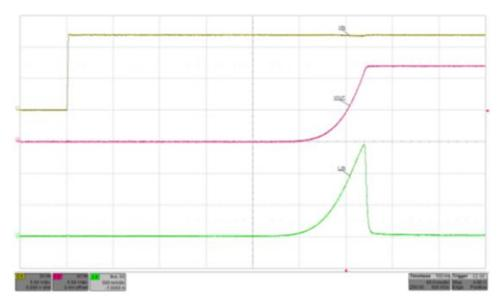
Figure 15. Waveform Showing the Charge Up of 3.6 mF Holdup Capacitor with a Discrete Solution
