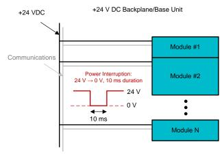
Figure 8. Illustration of Power Interruption Test (IEC 61000-4-29)
