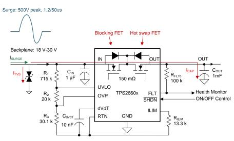
Figure 17. Simplified Schematic for Surge Protection
