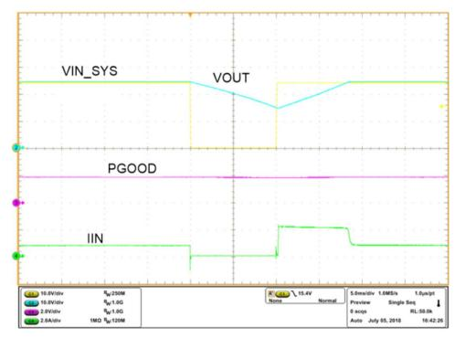
Figure 10. Waveform of TPS2663 in Response to 10 ms Power Interruption Test
