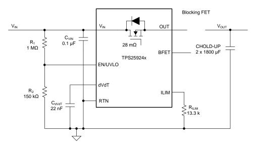
Figure 13. Simplified Schematic of Discrete Solution
