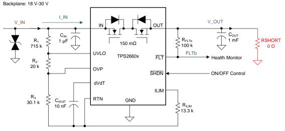
Figure 4. Simplified Schematic of TPS2660
