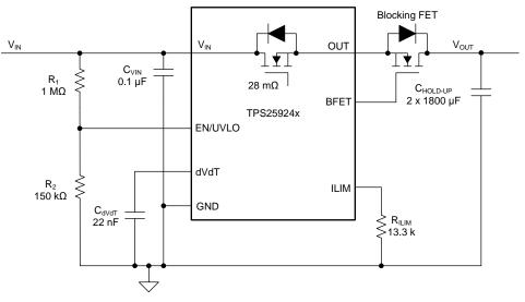
Figure 12. Simplified Schematic of the TPS25924x
