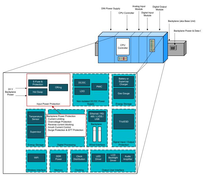
Figure 2. End Equipment Reference Diagram of PLC CPU Module
