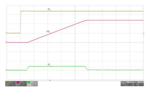
Figure 14. Waveform Showing the Charge Up of 3.6 mF Holdup Capacitor with the TPS25924x
