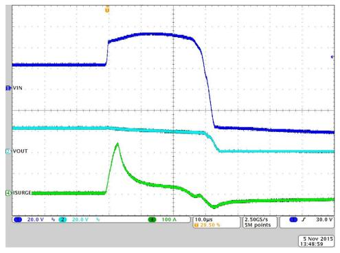
Figure 18. Waveform of TPS2660 During a 500 V / 2  $\Omega$  Surge Event
