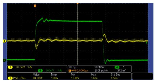
Figure 2-1. TPSM8A29 Load Transient
