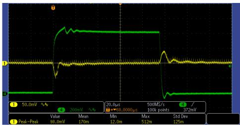
Figure 2-3. TPS543B20 Load Transient with 3 x 100-µF
