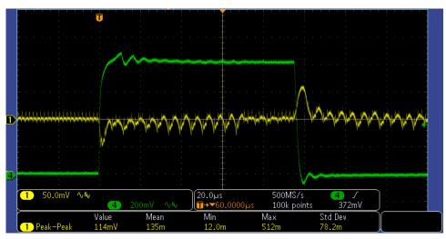
Figure 2-2. TPS543B20 Load Transient with 2 x 100-µF
