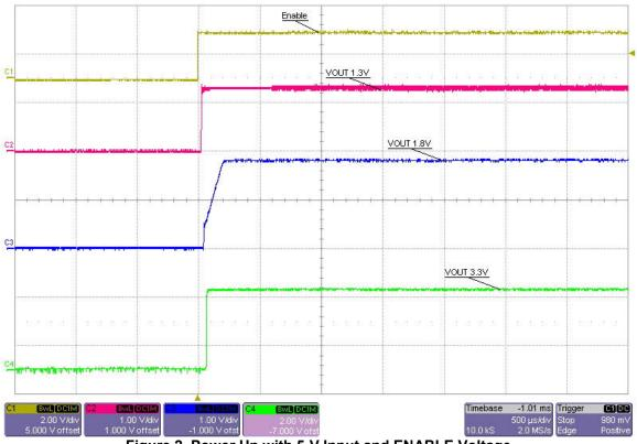
Figure 2. Power Up with 5-V Input and ENABLE Voltage
