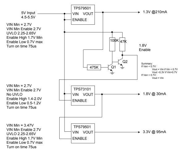
Figure 1. Block Diagram of Power Design
