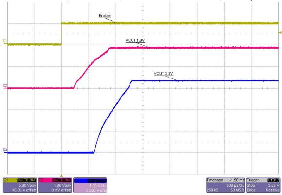
Figure 1. Power Up with 5-V Input and ENABLE Voltage
