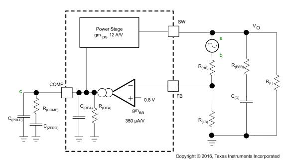
Figure 42. Small Signal Model for Loop Response
