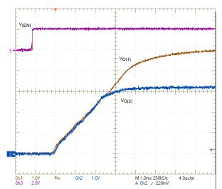
Figure 36. Simultaneous Startup With Tracking Resistor
