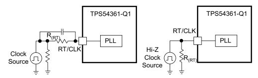
Figure 38. Synchronizing to a System Clock
