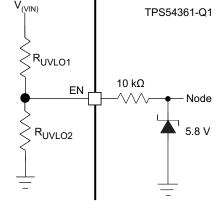
Figure 26. Adjustable Undervoltage Lockout (UVLO)
