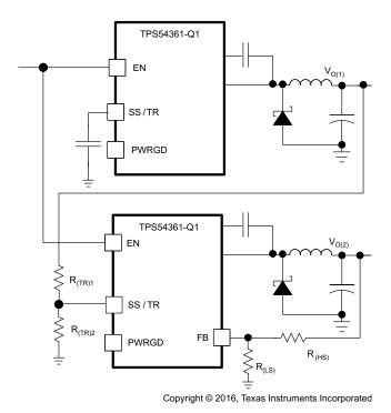
Figure 33. Schematic for Ratiometric and Simultaneous Start-Up Sequence
