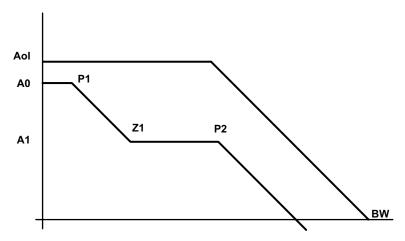
Figure 45. Frequency Response of the Type 2A and Type 2B Frequency Compensation
