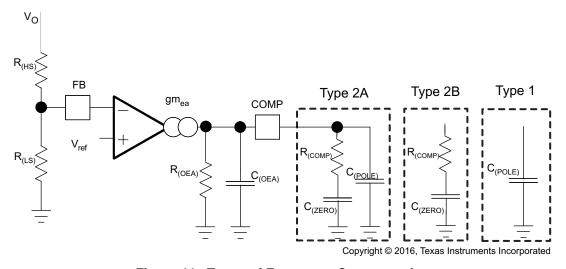
Figure 44. Types of Frequency Compensation
