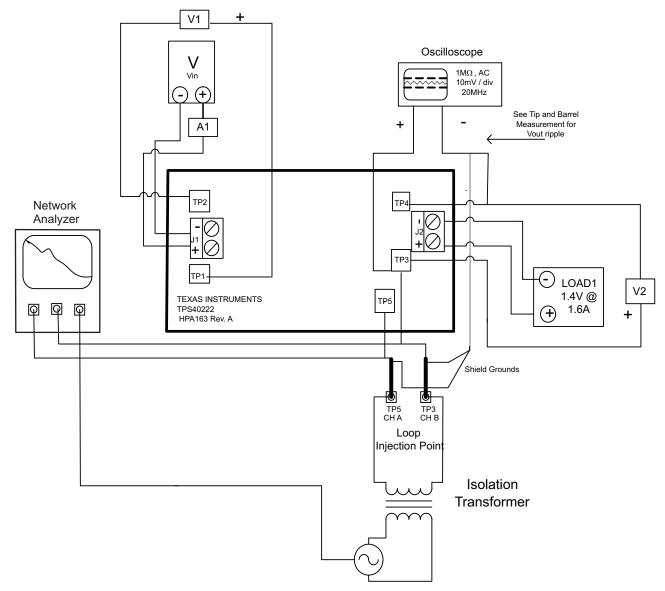
Figure 4. Control Loop Measurement Setup
