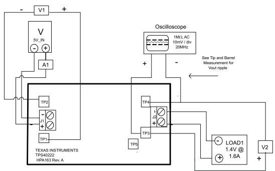
Figure 2. TPS40222EVM-001 Recommended Test Setup
