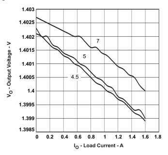
Figure 6. TPS402222EVM-001 Line and Load Regulation
