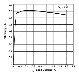
Figure 5. TPS40222EVM-001 Efficiency 1.4 V Out ( $V_{5V\_IN} = 4.5-8$  V,  $V_{1V4\_OUT} = 1.4$  V,  $I_{1V5\_OUT} = 0-1.6$  A)
