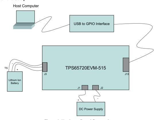
Figure 2. Hardware Board Connection
