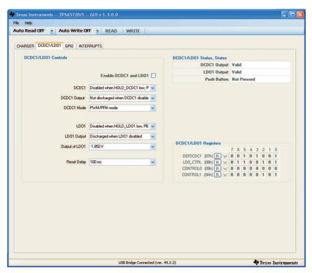
Figure 5. Software DCDC1/LDO1 View
