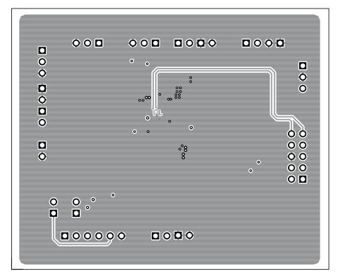
Figure 10. TPS65720EVM Bottom Copper (X-Ray View )
