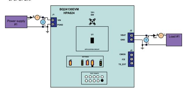
Figure 1. Original Test Setup for HPA624 (bq24130EVM)
