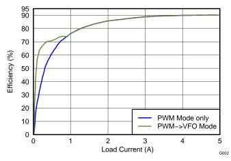
Figure 5. TPS23751EVM-104 DC/DC Converter Efficiency
