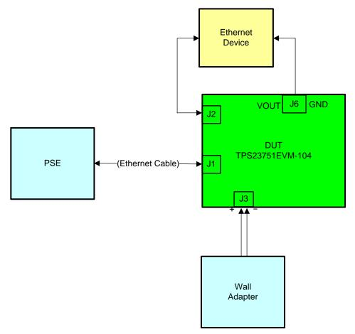
Figure 3. Typical TPS23751EVM-104 Test Setup
