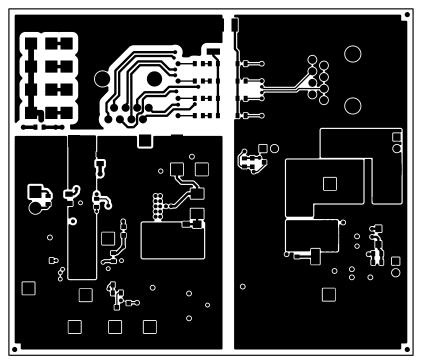
Figure 11. Bottom-Side Routing
