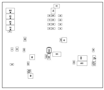
Figure 12. Bottom-Side Placement
