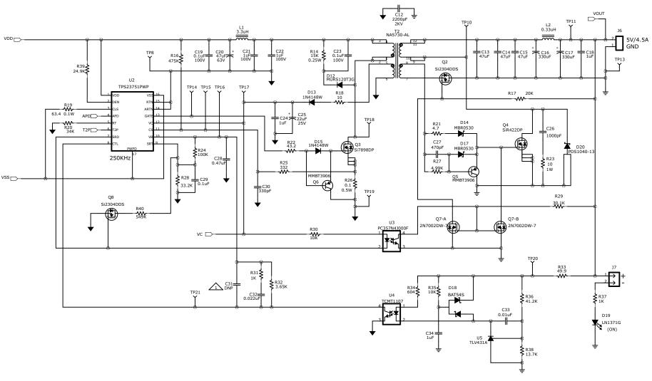
Figure 2. TPS23751EVM-104 Schematic (2 of 2)
