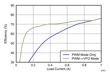
Figure 6. TPS23751EVM-104 DC/DC Converter Light-Load Efficiency
