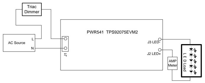
Figure 2. Dimming Wiring Diagram
