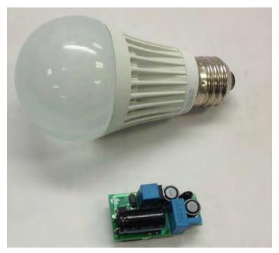
Figure 17. EVM Board and LED Bulb
