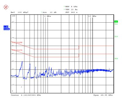
Figure 13. Conducted EMI Scan, 9 LEDs
