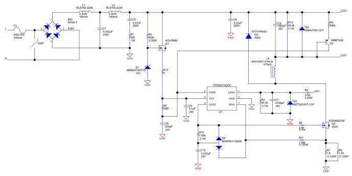
For VLED < 15 V, replace R13 with a diode (DFLS1200 or similar) and modify C5  $\ge$  22  $\mu$ F.
