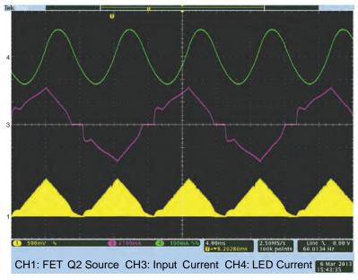
Output Ripple (V<sub>OUT</sub>: 26.2 V, I<sub>OUT</sub> 380 mA, THD 13.8%)
