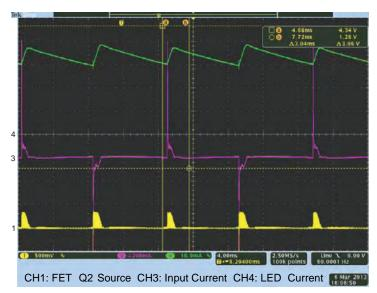
Figure 10. Leviton Leading-Edge 6684, Output = 20 mA,  $V_{LED}$  = 26 V
