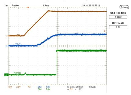
Figure 7. TPS57112EVM Startup Relative to VIN
