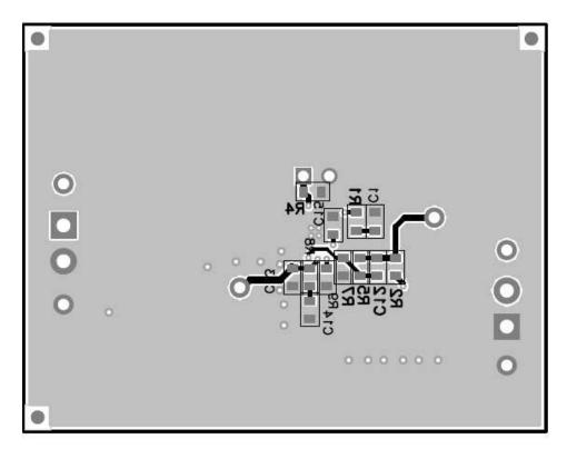
Figure 12. TPS57112EVM Bottom-Side Assembly
