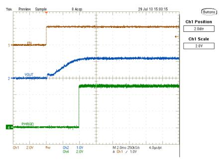
Figure 8. TPS57112EVM Startup Relative to Enable
