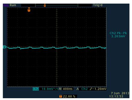
Figure 6. TPS57112EVM Output Ripple
