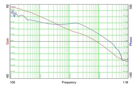
Figure 5. TPS57112EVM Loop-Response Measurement
