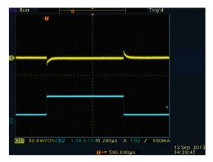
Figure 4. TPS57112EVM Load Transient
