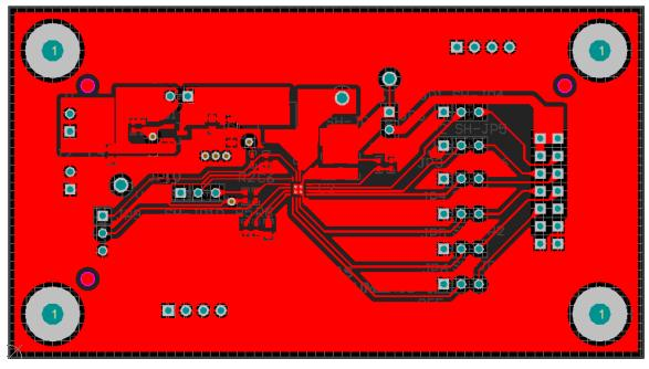
Figure 7. Top-Layer Routing
