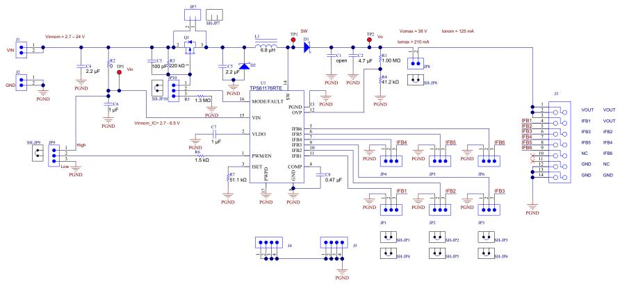
Figure 9. TPS61176EVM Schematic
