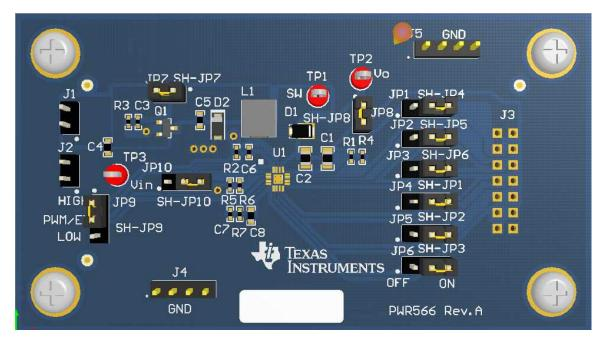
Figure 1. Default Configuration of Jumpers
