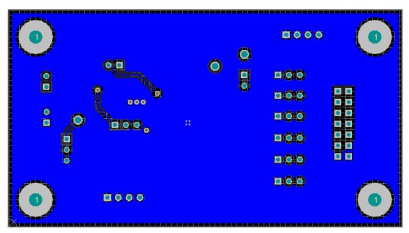
Figure 8. Bottom-Layer Routing
