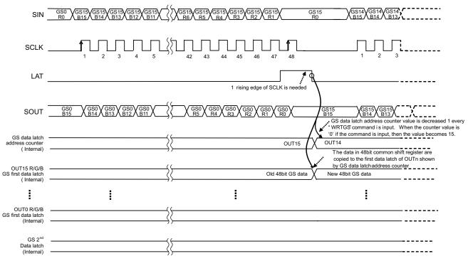
Figure 9. 48-Bit GS Data Write (WRTGS) Command in Traditional Trans Mode
