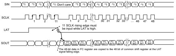
Figure 26. FC Data Read (READFC) Command
