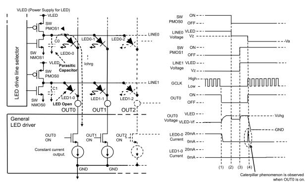
Figure 28. LED Caterpillar Phenomenon Mechanism
