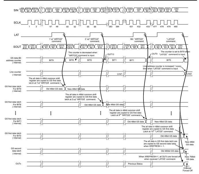
Figure 15. GS Data Write Sequence (9 "WRTGS" + 1 "LATGS" command) in Poker Mode
