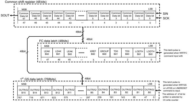
Figure 6. Common Shift Register and Data Latch Configuration
