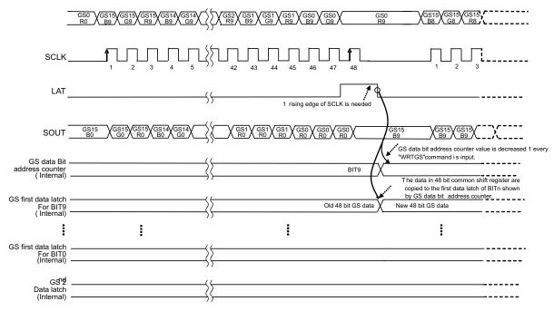
Figure 13. 48-Bit GS Data Write (WRTGS) Command in Poker Mode
