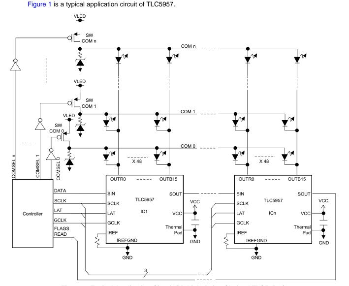
Figure 1. Typical Application Circuit (Multiple Daisy-Chained TLC5957s)
