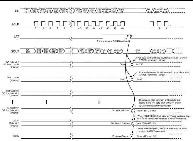
Figure 10. 768-Bit GS Data Latch (LATGS) Command in Traditional Trans Mode
