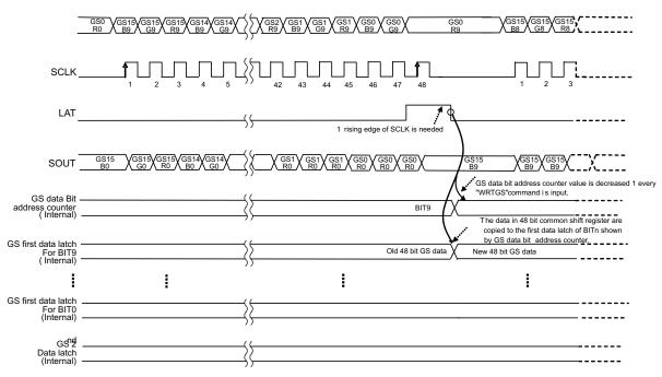
Figure 14. GS Data Latch (LATGS) Command in Poker Mode
