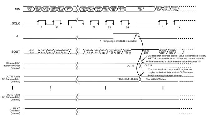
Figure 29. WRTGS Command at Double SCLK Mode
