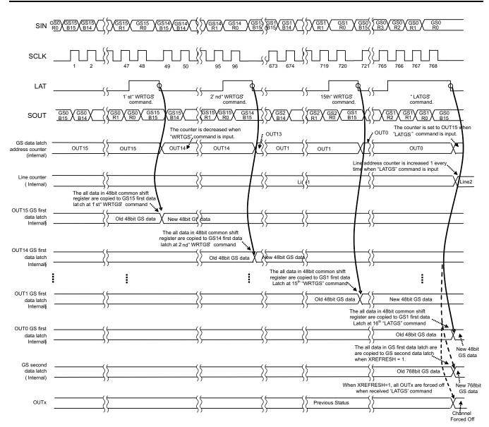
Figure 11. 768-Bit GS Data Write Sequence (15 times of "WRTGS" + 1 times of "LATGS" command)
