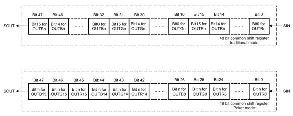
Figure 12. Traditional Mode vs Poker Mode Register
