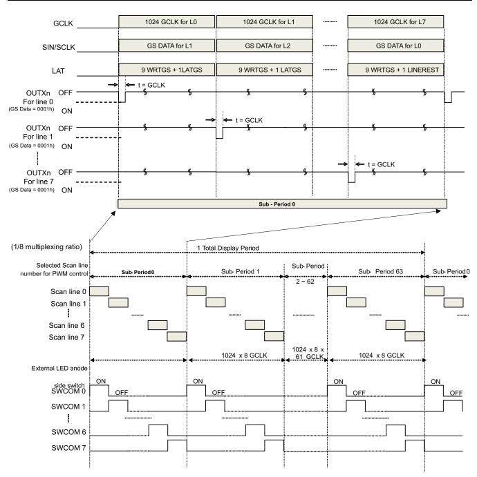
Figure 21. Whole Operation Sequence in 10-Bit Poker Mode
