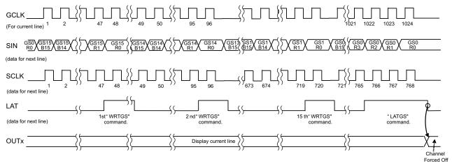
Figure 18. GS Data Writing in Multiplexing Application
