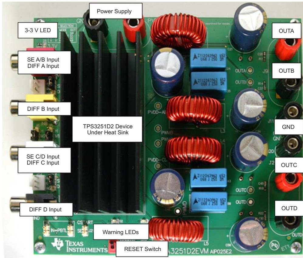
**Figure 2. TPA3251D2EVM Connections**
