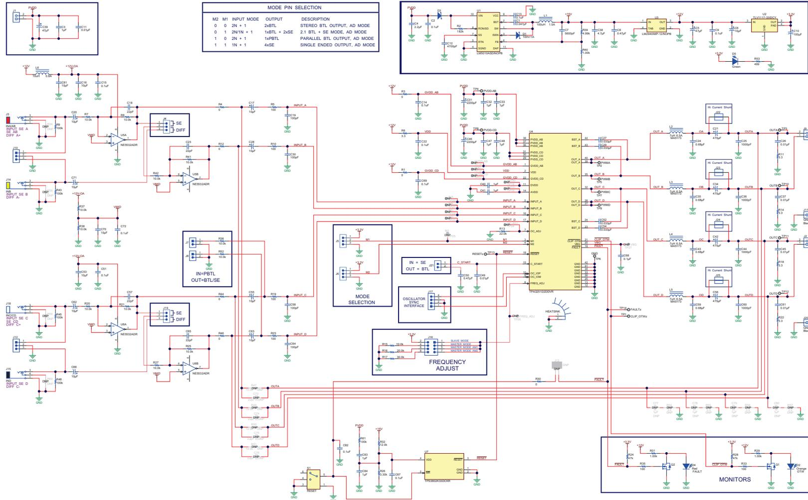
Figure 6. TPA3251D2EVM Schematic
