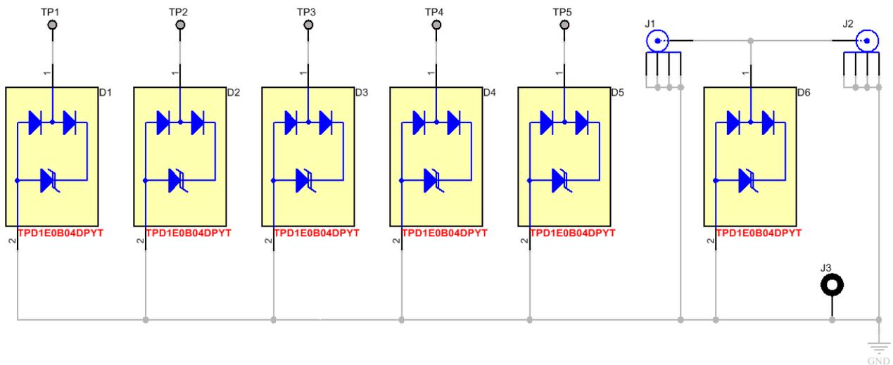
Figure 4. TPD1E0B04DPYEVM Schematic
