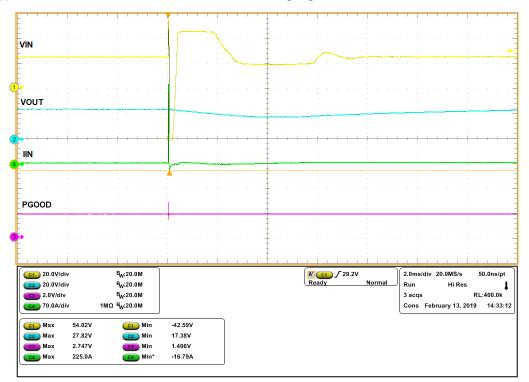
Figure 4. +500-V Surge Protection [C<sub>OUT</sub> = 2 mF, R<sub>LOAD</sub> = 6  $\Omega$ , VIN = 24 V, I<sub>LIM</sub> = 4.5 A, Peak Pulse Power = 12 kW]
