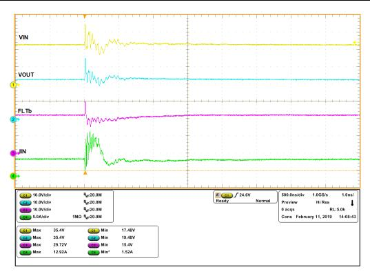
Figure 6. +2-kV EFT Protection [C<sub>OUT</sub> = 1  $\mu$ F, R<sub>LOAD</sub> = 4.8- $\Omega$ , VIN = 24 V, I<sub>LIM</sub> = 6 A]
