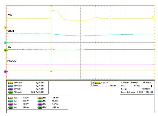
Figure 5. –500-V Surge Protection [ $C_{OUT}$  = 2 mF,  $R_{LOAD}$  = 6  $\Omega$ , VIN = 24 V,  $I_{LIM}$  = 4.5 A, Peak Pulse Power = 9.4 kW]
