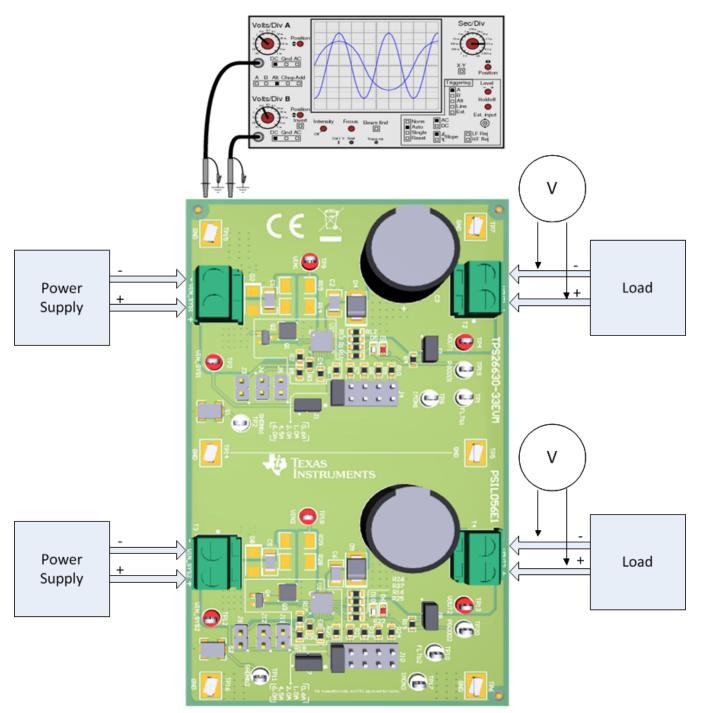
Figure 1. EVM Test Setup
