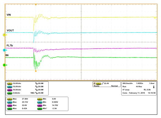
Figure 7. –2-kV EFT Protection [C<sub>OUT</sub> = 1  $\mu$ F, R<sub>LOAD</sub> = 4.8  $\Omega$ , VIN = 24 V, I<sub>LIM</sub> = 6 A]
