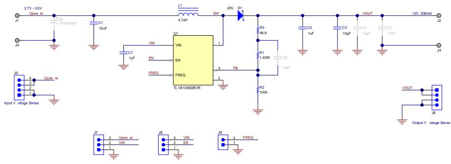
Figure 1. TLV61048EVM-042 Schematic
