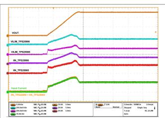
Figure 5-4. Start-up Profile with ENABLE: Current Sharing between TPS25990 and TPS25985 eFuses (V<sub>IN</sub> = 12 V, EN Stepped Up from 0 V to 3 V, C<sub>OUT</sub> = 15.47 mF, R<sub>LOAD</sub> = 0.4  $\Omega$ , R<sub>ILIM(TPS25990)</sub> = 523  $\Omega$ , R<sub>ILIM(TPS25985)</sub> = 402  $\Omega$ , V<sub>IREF</sub> = 1 V, and C<sub>DVDT</sub> = 33 nF)
