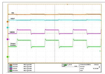
Figure 5-9. Transient Overload Performance in TPS25990EVM ( $V_{IN}$  = 12 V,  $t_{ITIMER}$  = 20 ms,  $C_{OUT}$  = 470  $\mu$ F,  $R_{IMON}$  = 1.47  $\parallel$  1.1  $k\Omega$ ,  $V_{IREF}$  = 1 V,  $I_{OUT}$  Ramped from 85 A to 140 A then 85 A within 15 ms)
