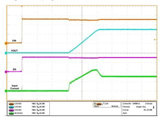
Figure 5-2. Hot Plug Profile with TPS25990 eFuse and TPS25985 eFuse in Parallel (V<sub>IN</sub> Stepped Up from 0 V to 12 V,  $C_{OUT}$  = 15.47 mF,  $C_{DVDT}$  = 33 nF,  $R_{ILIM(TPS25990)}$  = 523  $\Omega$ ,  $R_{ILIM(TPS25985)}$  = 402  $\Omega$ ,  $V_{IREF}$  = 1 V, and  $R_{LOAD}$  = 0.4  $\Omega$ )
