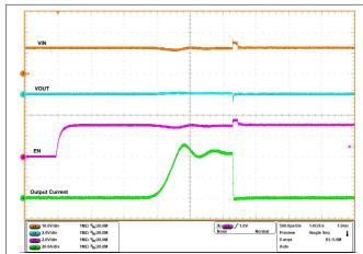
Figure 5-6. Power Up into Output Short Response in TPS25990EVM ( $V_{IN}$  = 12 V, EN Stepped Up from 0 V to 3 V,  $R_{ILIM(TPS25990)}$  = 665  $\Omega$ ,  $R_{ILIM(TPS25985)}$  = 499  $\Omega$ ,  $V_{IREF}$  = 1 V, and OUT Shorted to PGND)
