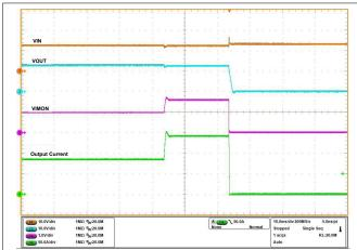
Figure 5-11. Overcurrent Performance in TPS25990EVM ( $V_{IN}$  = 12 V,  $t_{ITIMER}$  = 20 ms,  $C_{OUT}$  = 470  $\mu$ F,  $R_{IMON}$  = 1.47  $\parallel$  1.1  $k\Omega$ ,  $V_{IREF}$  = 1 V,  $I_{OUT}$  Ramped from 85 A to 140 A then 85 A within 30 ms)
