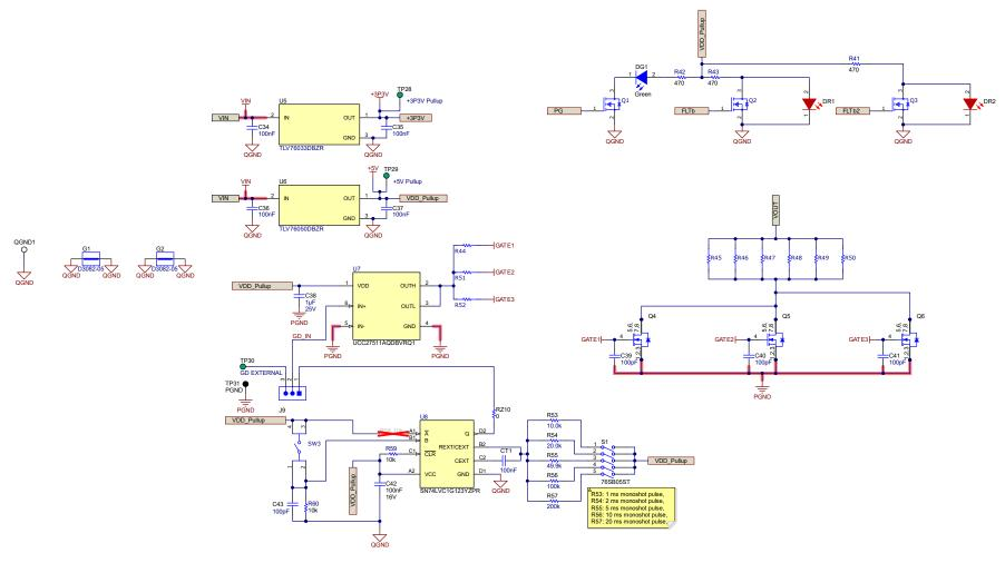
Figure 3-1. TPS25990EVM eFuse Evaluation Board Schematic
