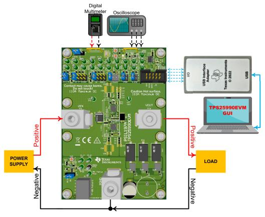
Figure 5-1. TPS25990EVM Setup with Test Equipment
