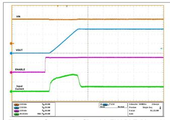
Figure 5-3. Start-up Profile with ENABLE ( $V_{IN}$  = 12 V, EN Stepped Up from 0 V to 3 V,  $C_{OUT}$  = 18.47 mF,  $R_{LOAD}$  = 1.2  $\Omega$ ,  $R_{ILIM(TPS25990)}$  = 523  $\Omega$ ,  $R_{ILIM(TPS25985)}$  = 402  $\Omega$ ,  $V_{IREF}$  = 1 V, and  $C_{DVDT}$  = 33 nF)
