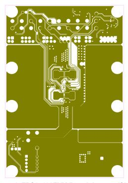
Figure 7-8. TPS25990EVM Board: Layer 5 (Signal)
