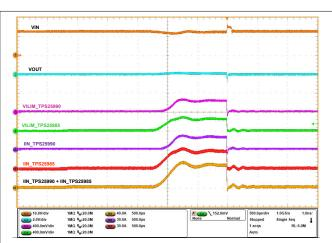
Figure 5-7. Power Up into Output Short Response in TPS25990EVM: Current Sharing between TPS25990 and TPS25985 eFuses (V<sub>IN</sub> = 12 V, EN Stepped Up from 0 V to 3 V, R<sub>ILIM(TPS25990)</sub> = 665 Ω, R<sub>LIMI(TPS25985)</sub> = 499 Ω, V<sub>IREF</sub> = 1 V, and OUT Shorted to PGND)
