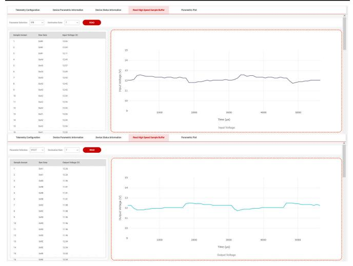
Figure 6-17. TPS25990EVM-GUI: Device Telemetry: Read High Speed Sample Buffer: Input and Output Voltages
