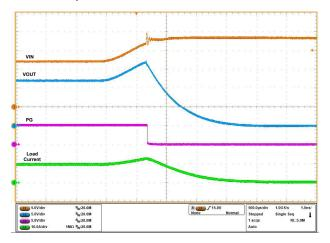
Figure 5-8. Overvoltage Lockout Response of TPS25990 eFuse ( $V_{IN}$  Ramped Up from 12 V to 18 V,  $C_{OUT}$  = 470  $\mu$ F, and  $R_{LOAD}$  = 1.2  $\Omega$ )
