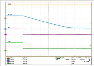
Figure 5-16. QOD Enabled on TPS25990 eFuse ( $V_{IN}$  = 12 V,  $C_{OUT}$  = 470  $\mu$ F, and EN Pulled Low to 0.8 V)
