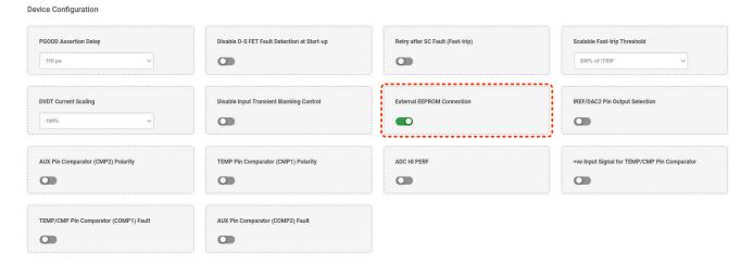
Figure 6-22. TPS25990EVM-GUI: Device Configuration: External EEPROM Connection
