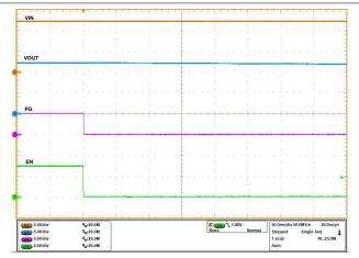
Figure 5-17. QOD Disabled on TPS25990 eFuse ( $V_{IN}$  = 12 V,  $C_{OUT}$  = 470  $\mu$ F, and EN Pulled Low to 0 V)
