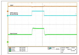
Figure 5-13. Transient Overload Performance in TPS25990EVM Using the Onboard Switching Circuit ( $V_{IN}$  = 12 V,  $t_{ITIMER}$  = 14 ms,  $C_{OUT}$  = 1470  $\mu$ F,  $R_{IMON}$  = 1.47  $\parallel$  1.1 k $\Omega$ ,  $V_{IREF}$  = 1 V,  $I_{OUT(Steady-State)}$  = 85 A, and  $I_{OUT(Transient)}$  = 65 A for 9 ms)
