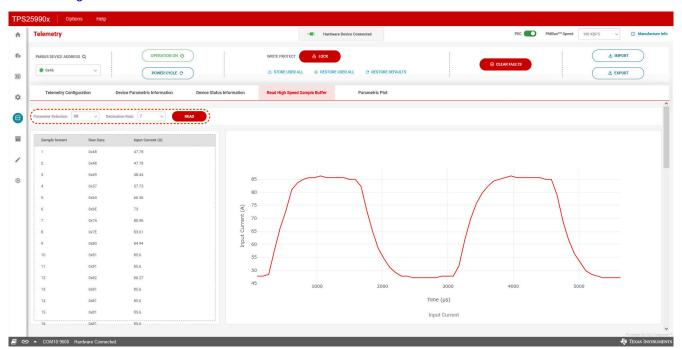
Figure 6-16. TPS25990EVM-GUI: Device Telemetry: Read High Speed Sample Buffer: Input Current
