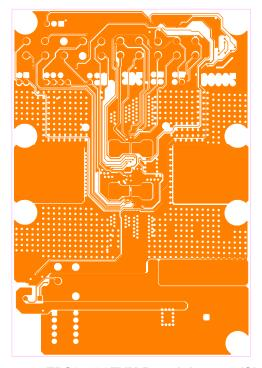
Figure 7-7. TPS25990EVM Board: Layer 4 (Signal)
