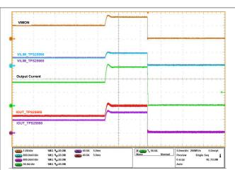
Figure 5-12. Overcurrent Performance in TPS25990EVM: Current Sharing between TPS25990 and TPS25985 eFuses (V<sub>IN</sub> = 12 V, t<sub>ITIMER</sub> = 10 ms, C<sub>OUT</sub> = 470 μF, R<sub>IMON</sub> = 1.47 || 1.1 kΩ, V<sub>IREF</sub> = 1 V, I<sub>OUT</sub> Ramped from 85 A to 140 A then 85 A within 15 ms)
