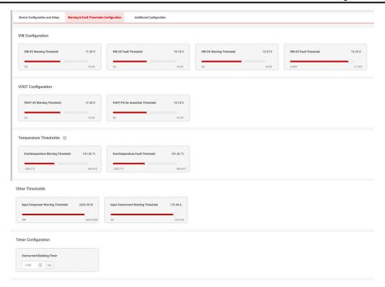
Figure 6-8. TPS25990EVM-GUI: Device Configuration: Warning & Fault Thresholds Configuration
