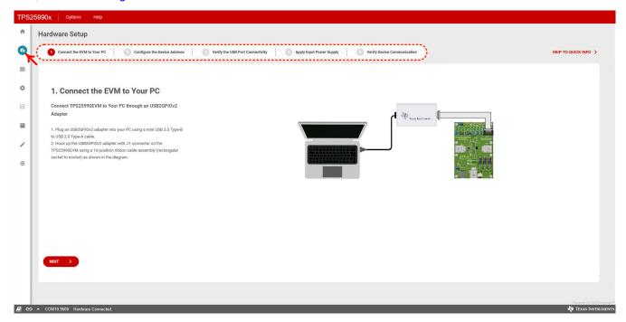
Figure 6-3. Hardware Setup: Establishing the Communication Between the EVM and GUI
