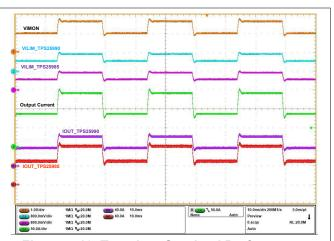
Figure 5-10. Transient Overload Performance in TPS25990EVM: Current Sharing between TPS25990 and TPS25985 eFuses (V<sub>IN</sub> = 12 V, t<sub>ITIMER</sub> = 20 ms, C<sub>OUT</sub> = 470 μF, R<sub>IMON</sub> = 1.47 || 1.1 kΩ, V<sub>IREF</sub> = 1 V, I<sub>OUT</sub> Ramped from 85 A to 140 A then 85 A within 15 ms)
