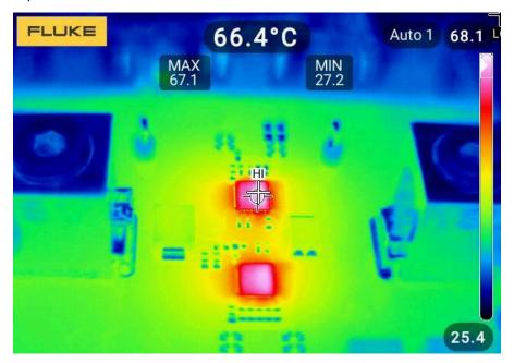
Figure 5-18. Thermal Performance in TPS25990EVM ( $V_{IN}$  = 12 V,  $R_{IMON}$  = 0.91 || 1.1 k $\Omega$ ,  $V_{IREF}$  = 1.13 V, and  $I_{OUT}$  = 110 A)
