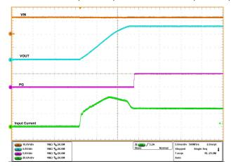
Figure 5-5. Start-up with Current Limit Response in TPS25990EVM ( $V_{IN}$  = 12 V, EN Stepped Up from 0 V to 3 V,  $R_{ILIM(TPS25990)}$  = 665  $\Omega$ ,  $R_{LIMI(TPS25985)}$  = 499  $\Omega$ ,  $V_{IREF}$  = 1 V,  $C_{OUT}$  = 18.47 mF,  $R_{LOAD}$  = 0.45  $\Omega$ , and  $C_{DVDT}$  = 33 nF)
