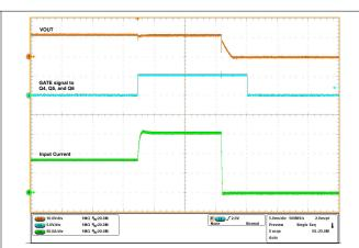
Figure 5-14. Persistent Overload Performance in TPS25990EVM Using the Onboard Switching Circuit (V<sub>IN</sub> = 12 V, t<sub>ITIMER</sub> = 14 ms, C<sub>OUT</sub> = 1470  $\mu$ F, R<sub>IMON</sub> = 1.47 || 1.1 k $\Omega$ , V<sub>IREF</sub> = 1 V, I<sub>OUT(Steady-State)</sub> = 85 A, and I<sub>OUT(Transient)</sub> = 65 A for 18 ms)
