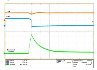
Figure 5-15. Output Hot Short Response in TPS25990EVM ( $V_{IN}$  = 12 V,  $R_{IMON}$  = 1.47 || 1.1 k $\Omega$ ,  $V_{IREF}$  = 1 V, and  $C_{OUT}$  = 10  $\mu$ F)
