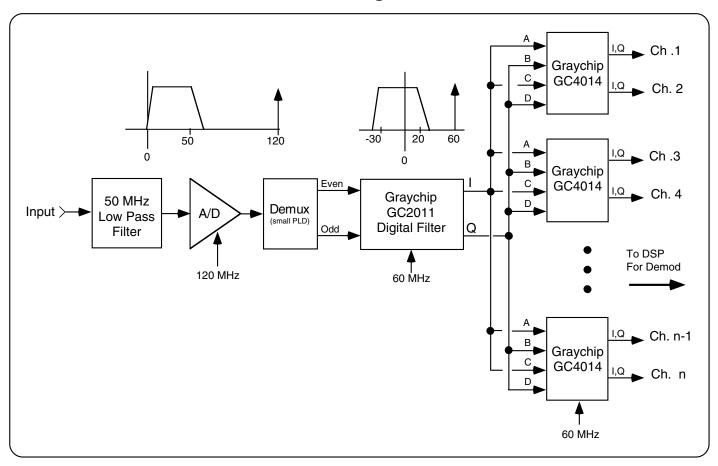
This application note describes how a 120 MHz sample rate multi-channel digital down-conversion system can be implemented using GRAYCHIP GC2011 Digital Filter and GC4014 Quad Digital Receiver chips.
