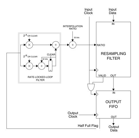
Figure 1. Resampler in RLL Mode
