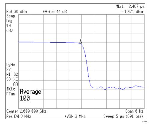
Figure 4. Output Power vs Time During Power-Off Operation (5 V to 0 V)
