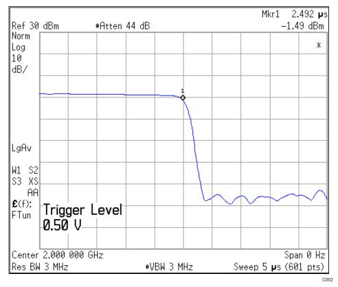
Figure 2. Output Power vs Time With VccLO Power-Off Operation (From 5 V to 0 V)
