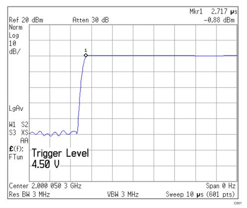
Figure 1. Output Power vs Time With VccLO Power-On Operation (From 0 V to 5 V)
