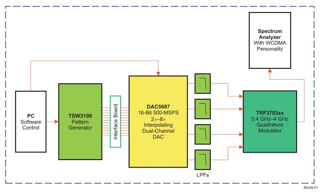
Figure 3. ACPR Test Setup for DAC5687 and TRF3703xx
