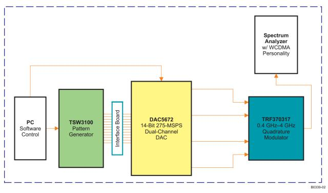
Figure 10. ACPR Test Setup for DAC56x2 and TRF3703xx
