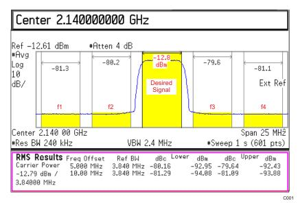
Figure 1. ACPR Spectral Representation of Modulated (Desired) and Adjacent Channels
