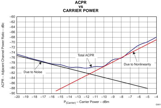
Figure 2. ACPR Performance of Single-Carrier WCDMA Signal Using DAC5687 and TRF370317 vs Carrier Power
