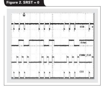
it is not appropriate to consider the SYNC pulse as an interrupt source to the host processor. The SYNC pulse is merely an indication that data currently available is the data acquired from channel 1.
